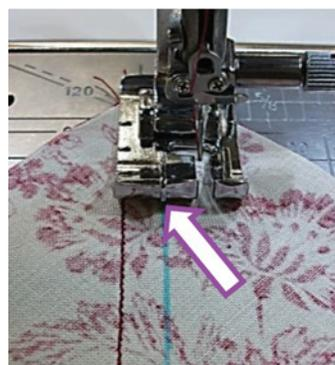
Match the 1/4" guide line with the mark and sew. As the guide line is raised, it is easy to align with the mark.
