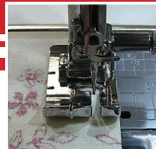
The 1/4" Seam Foot with no guide plate attached is a very useful tool for various types of piecing work. As with the 1/4" seam foot, you can sew the 1/4" position by aligning the cloth with the edge of the presser foot. While the guide is useful for lining up layers of fabric, not having a guide can be better for sewing on top of fabric like when making flying geese or half square triangles.
