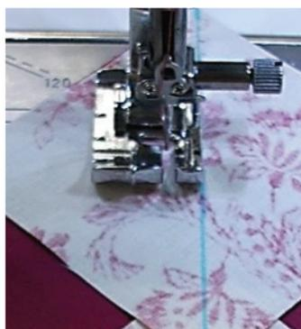
Align the edge of foot with the mark and sew.
